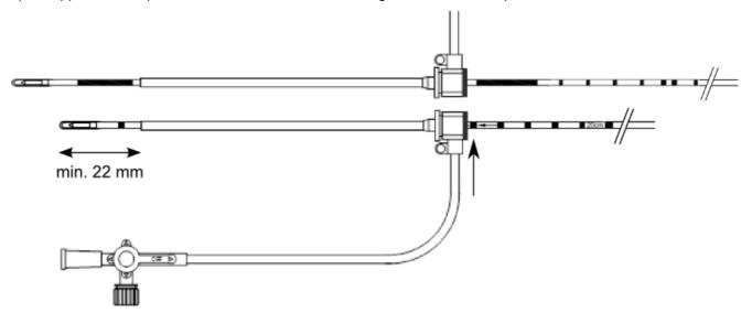
For the use of the LGO-Saturn Slight Side Fiber and LGO-Fistula Probe in cannulas, marking lines are applied at intervals of 5 mm and 10 mm. Prior to treatment make yourself familiar with your selected cannula.
