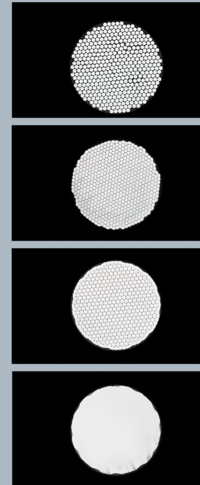
*With the glued bundle technology (GB), many fibers are glued together with an epoxy resin adhesive.*
