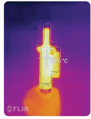
CFB 2.5mm input after continuous operation at 300W, CW, VIS moment after disconnected from source, >2h operation, no forced cooling. Thermal image displays that temperature of metal ferrule is below temperature of a human hand.
