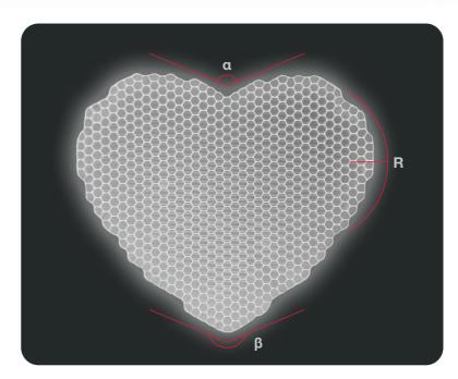
Inner angle ( $\alpha$ ), outer angle ( $\beta$ ) and curvature (R) structures are possible
