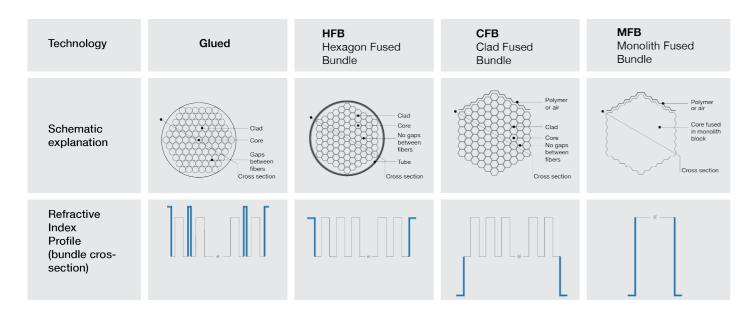
In the HFB design, the refractive index of the silica tube is higher than F-doped silica cladding of the individual fibers. In the CFB and MFB designs the fused fibers have a high refractive index cores and the outer layer of bundle is made of a low refractive index polymer or air.
