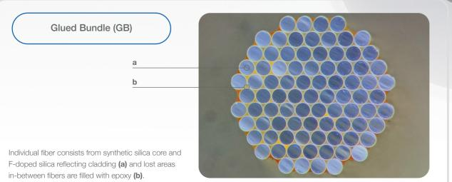
This is a simple technology where many fibers are glued together with epoxy glue. There are gaps between fibers caused by the circular shape of individual fibers and packing efficiency. The typical fill factor is around 0.85. Many companies can produce them in different degrees of quality. This is a cost-effective solution when maximum coupling is not required for the bundle outputs.
