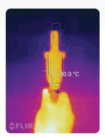
CFB output after continuous operation at 700W, CW, VIS moment after disconnected from source, >2h operation, no forced cooling. Thermal image displays that temperature of metal ferrule is slightly higher than temperature of a human hand.
