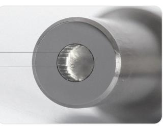
Comparing CFB and MFB, there the main difference is that fiber clads are removed and the fiber cores are fused together making one monolith body. There are no individual fibers that can be recognized. This type of fused bundle has the same advantages as CFB, however, there is a difference. MFB gives homogenous near field beam profile. MFB is ideal for low power applications, where homogenization is on the agenda.
